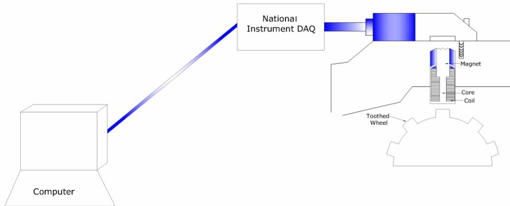
Figure 7.2 : Conceptual Diagram of Experimental Setup
