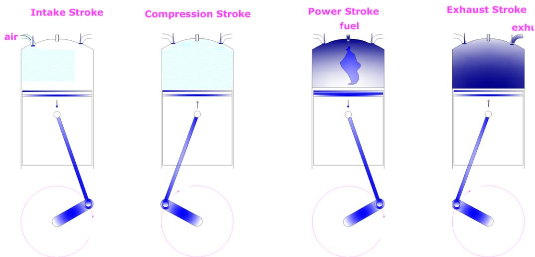
Figure 1.3 : Complete Ignition Cycle of SI Engine
