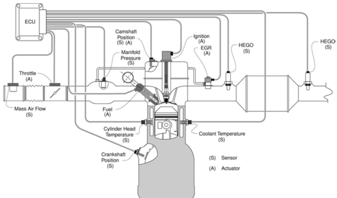
Figure 1.4 : Engine Cylinder connected with intake and exhaust manifold and sensors (*adopted from* . Cook J. A. et al, (2007, pp. 334 -335)
