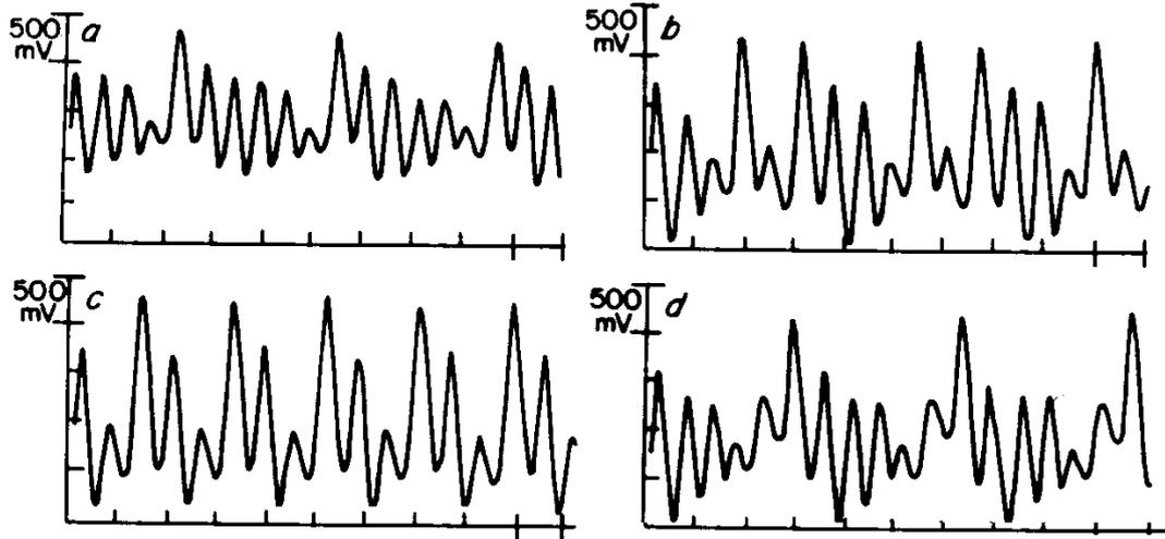
Figure 3.3 : Templates of engine speed patterns under different misfire conditions
