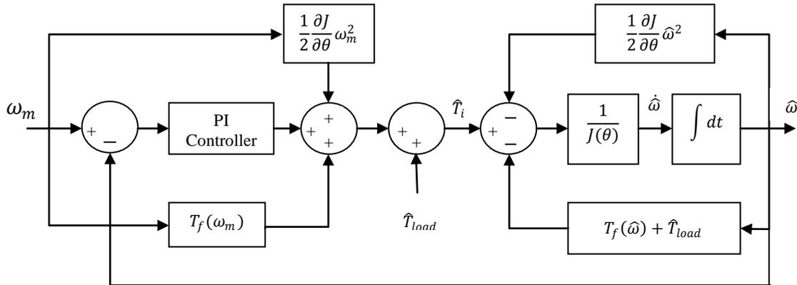
Figure 3.2 : Block diagram of PI feedforward indicated torque observer
