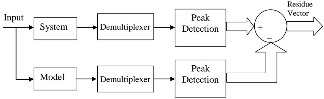
Figure 6.1 : Residual Generator with model running in Parallel
