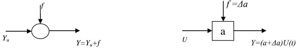
Figure 2.3 : (Left) Additive Fault (Right) Multiplicative Fault
