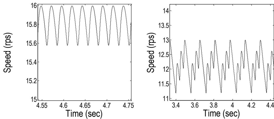
Fig. 7.1 Simulation Results: The waveforms representing fully balanced engine operation (left) one cylinder misfiring (right)
