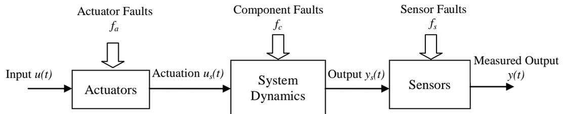
Figure 2.2: (Left) Actuator Fault (Middle) Component Fault (Right) Sensor Fault
