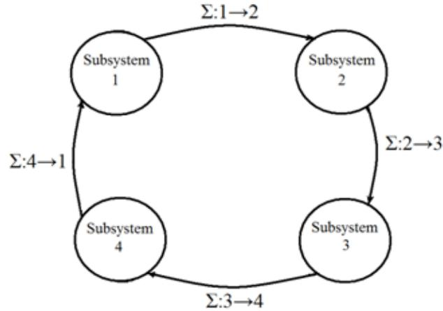
Figure 5.1 : Switching of subsystems (Adopted from Rizvi (2009, pp. 1-6))
