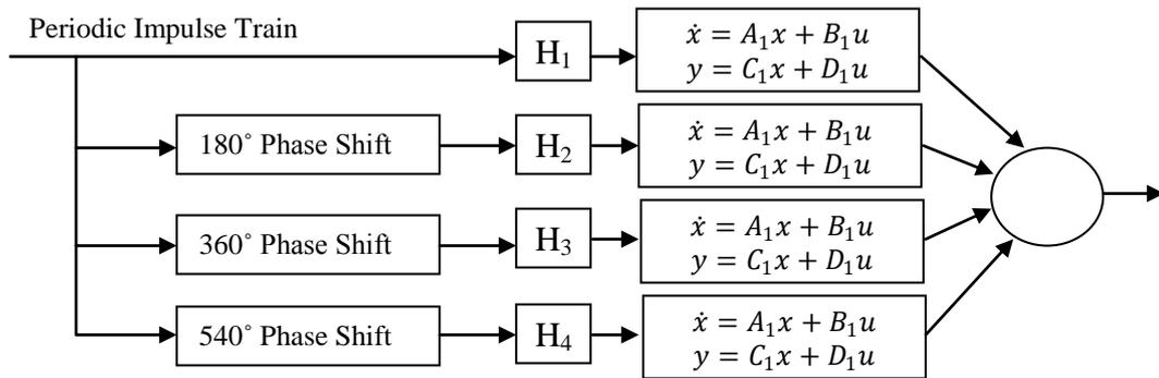
Figure 5.4: Block diagram for simple hybrid model of SI engine
