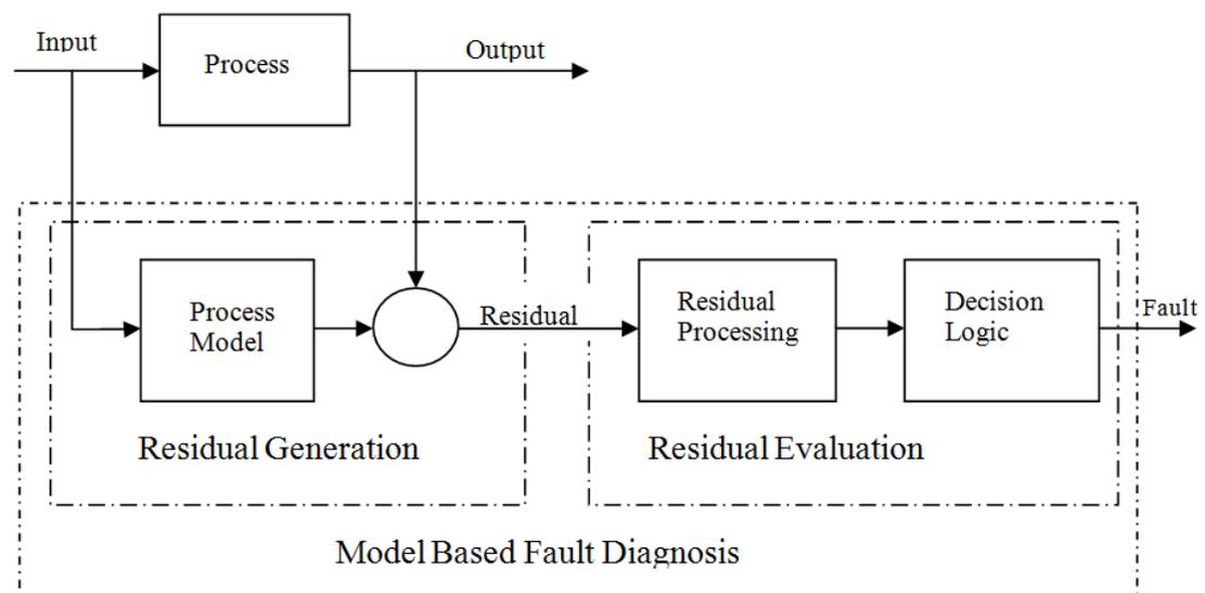
Figure 2.5 : Model Based Fault Diagnosis System
