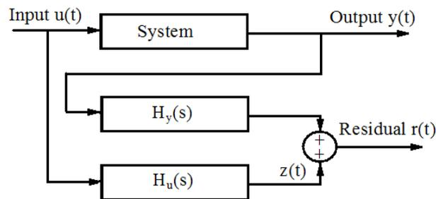
Figure 2.7 : General Structure of a Residual
