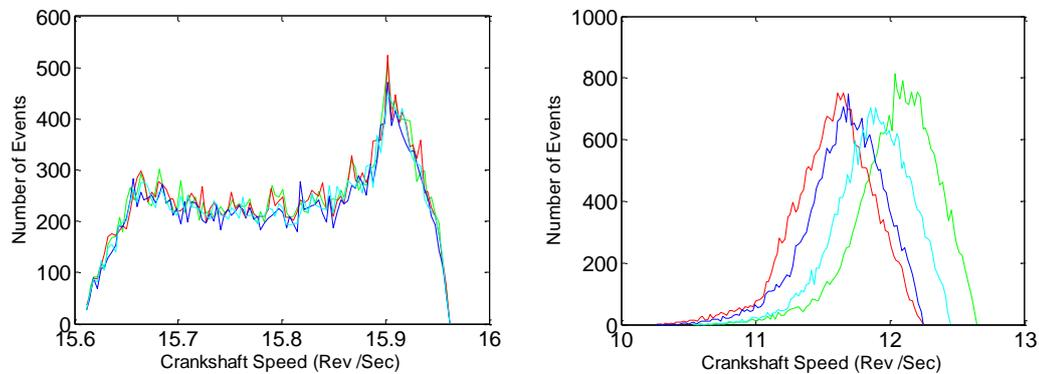
Figure 7.4 : Distribution of crankshaft speed during the activity period of four cylinders
