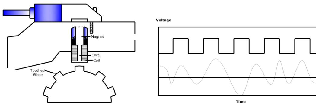
Figure 1.5 : (Left) Crankshaft Speed Sensor near gear teeth (Right) Sensor Signal
