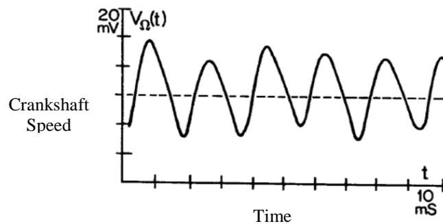
Figure 3.6 : Instantaneous Crankshaft Speed Signal as a function of time
