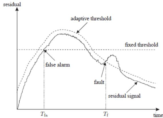
Figure 2.8 : Adaptive Threshold Selection
