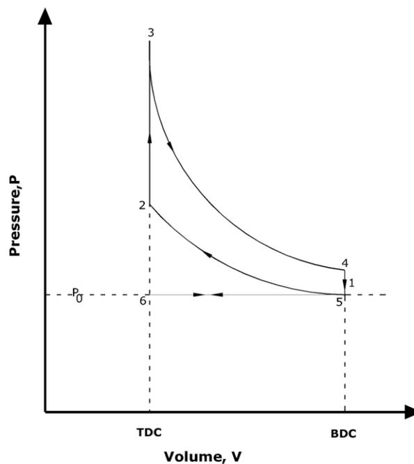
**Figure: PV Diagram of Otto Cycle**
