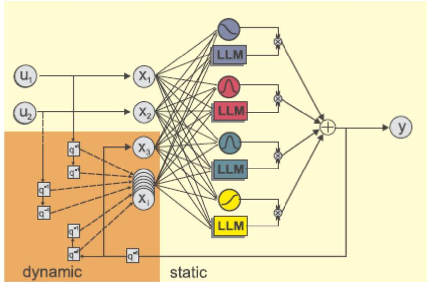
Figure 4.2 LOLIMOT net with external dynamics
