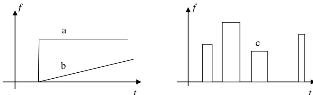
Figure 2.1: (Left) a. Abrupt Fault    b. Incipient Fault    (Right) Intermittent Fault
