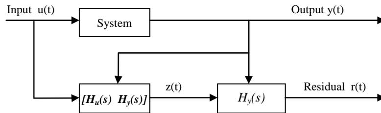
Figure 2.6 : Redundancy Signal Structure of a Residual Generator
