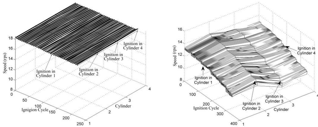
Figure 7.5 : Experimental Results: The surface representing cylinder 3 misfiring (left) no misfire (right) cylinder 3 misfiring
