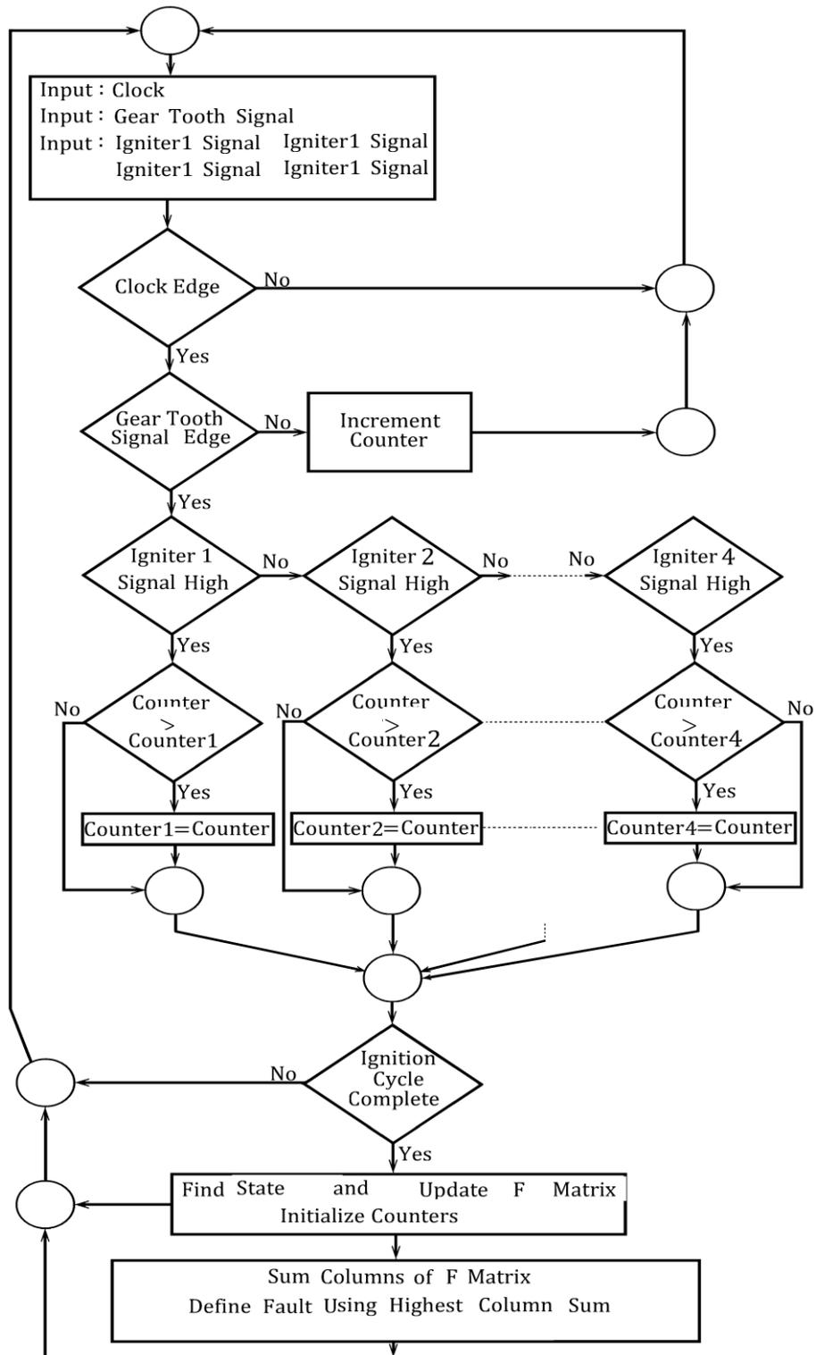
Figure 6.3: A Data based algorithm of Misfire detection for implementation in microcontroller
