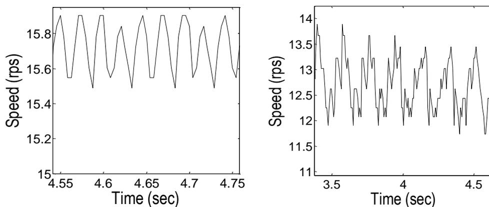
Figure 7.3 Experimental Results: The waveforms representing fully balanced engine operation (left) one cylinder misfiring (right)
