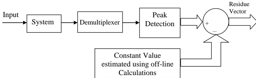
Figure 6.2: Simplified Residual Generator with off-line reference estimation
