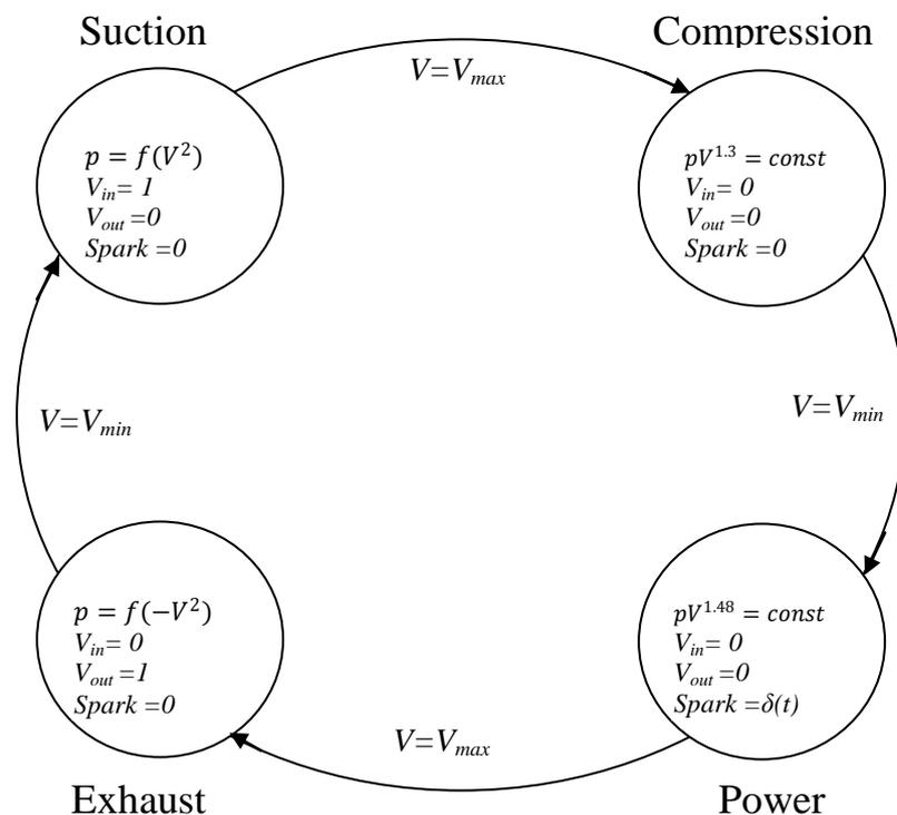
Figure 4.3: Engines Automaton with four States
