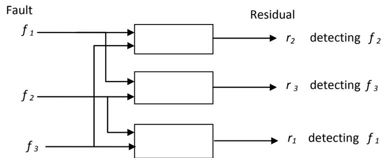
Figure 2.11 : Structured Residual Generator (Generalized Observer Scheme)
