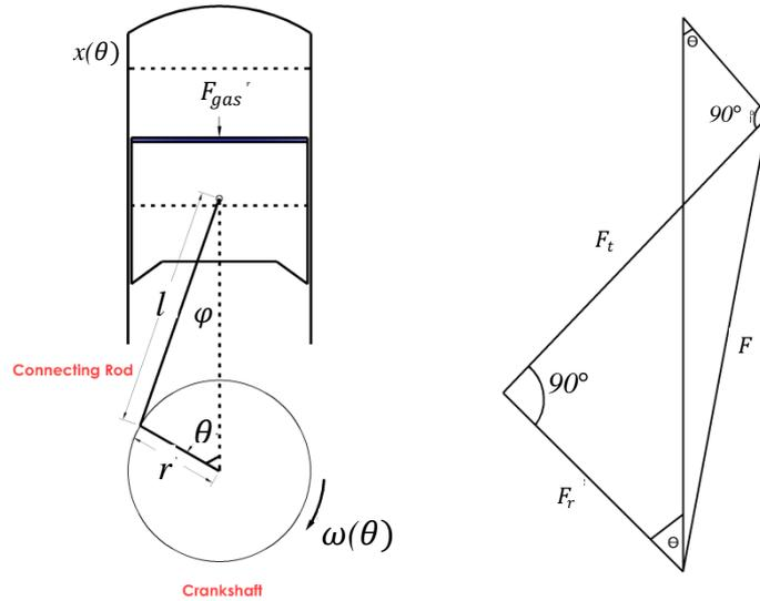
Figure 4.1: (a) Line Diagram of Crankshaft (b) Components of forces acting on crankshaft
