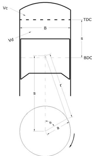
Figure 1.1: Line Diagram of Cylinder of SI Engine
