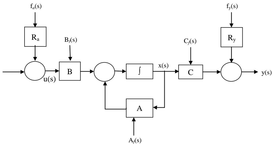
Figure 2.4 : System with Sensor, Actuator and System Faults
