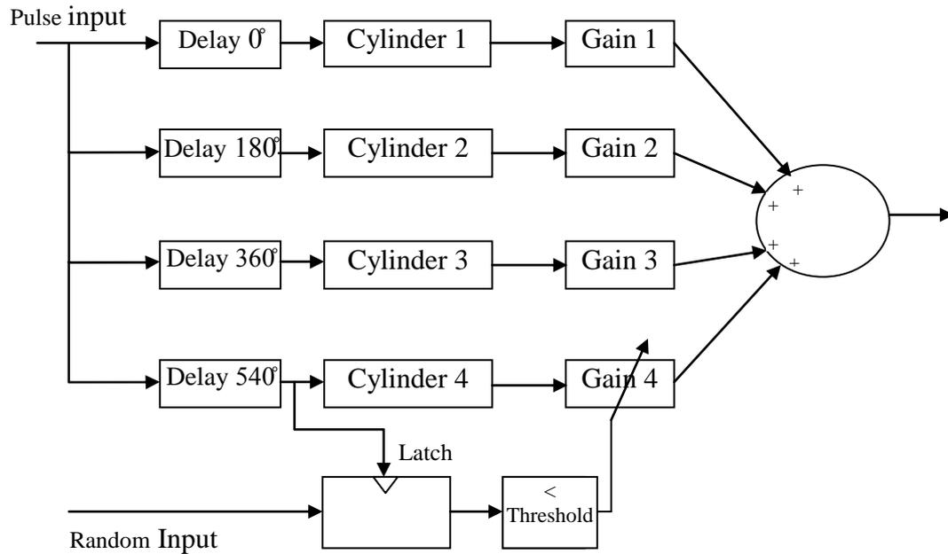
Figure 7.10 : Block Diagram of Experiment of Random Misfire
