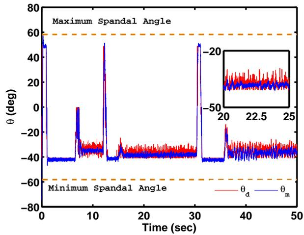
FIGURE 5.5: Desired and Measured angles for DC Servo Motor
