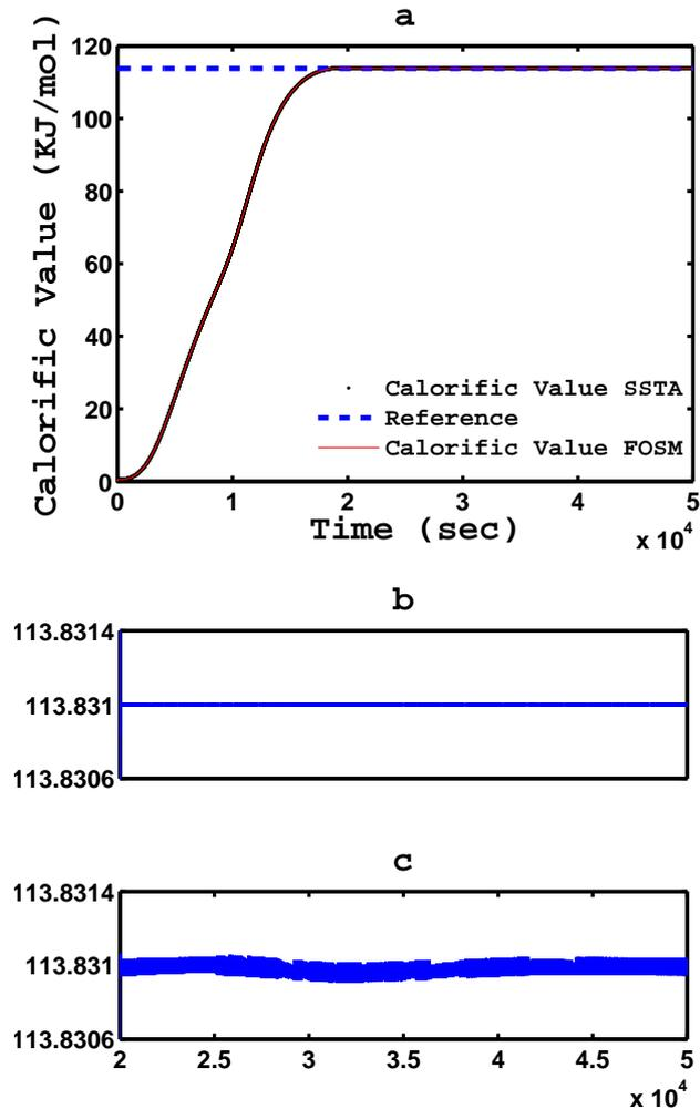
FIGURE 4.8: (a) Calorific value maintained by SSTA and FOSM controller. (b) Zoomed view of calorific value attained by SSTA. (c) Zoomed view of calorific value attained by FOSM controller
