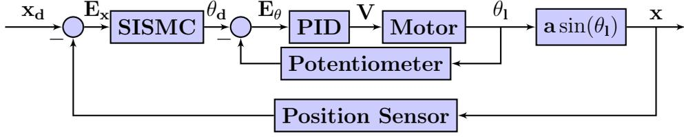
FIGURE 5.2: Control Configuration for Ball on a Beam Balancer
