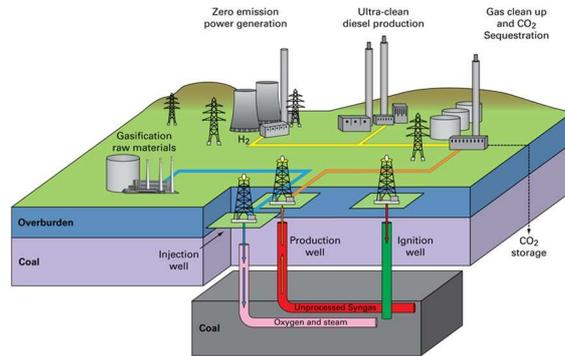
FIGURE 4.4: Underground Coal Gasification Reactor
