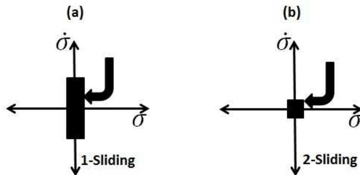
FIGURE 3.7: Description of Sliding Order and Manifold Dimension [1]
