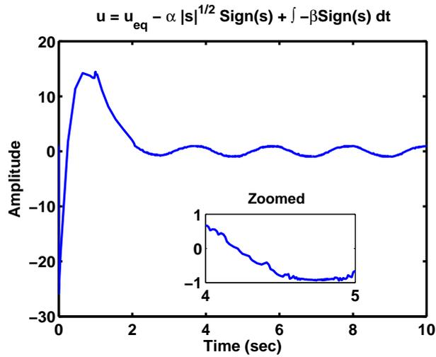
FIGURE 3.10: Controller effort produced by the STA in the presence of disturbance ( $\sin(3t)$ )
