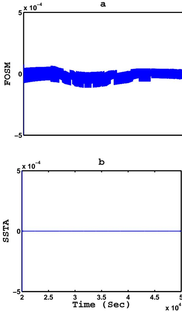
FIGURE 4.10: Sliding surface (error of output and reference) enforced by (a) FOSM (b) SSTA
