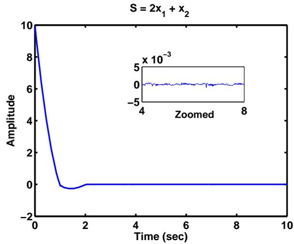
FIGURE 3.9: Sliding surface reached and maintained by STA
