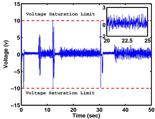
FIGURE 5.6: Voltage Applied to the DC Motor
