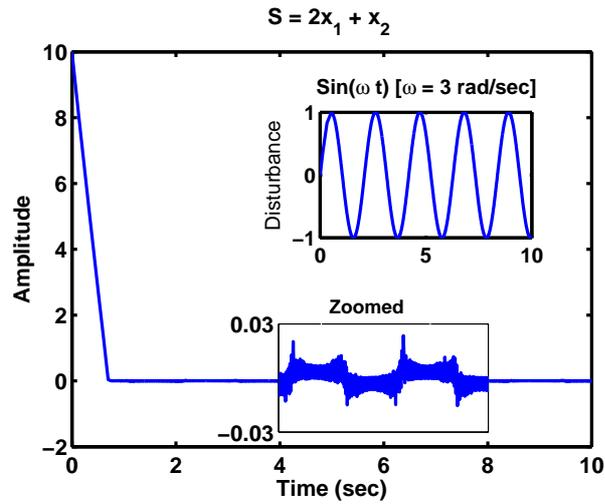
FIGURE 3.2: Sliding surface and the applied external disturbance
