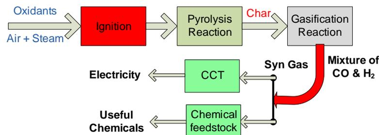
FIGURE 4.5: A Snapshot of the UCG process
