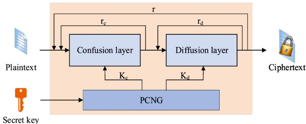
FIGURE 3.6: Structure of chaos based image encryption scheme
