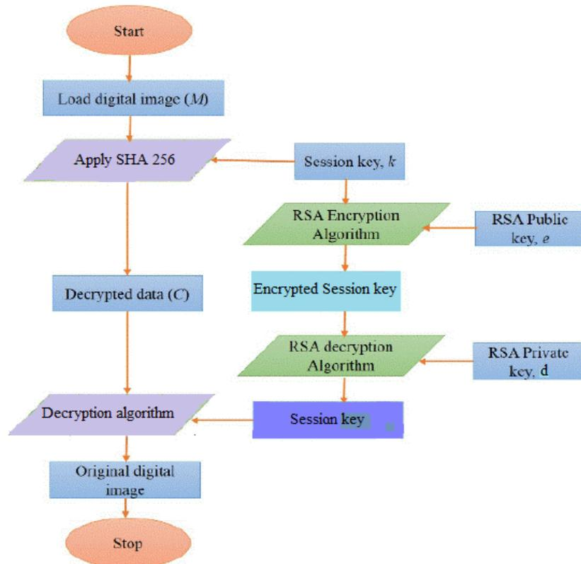
FIGURE 5.1: Flow diagram of the proposed cryptosystem
