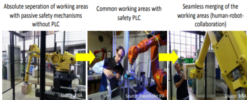
FIGURE 3.1: Evolution of Safe Human Robot Collaboration. Adapted with permission from Azfar Khalid [6].
