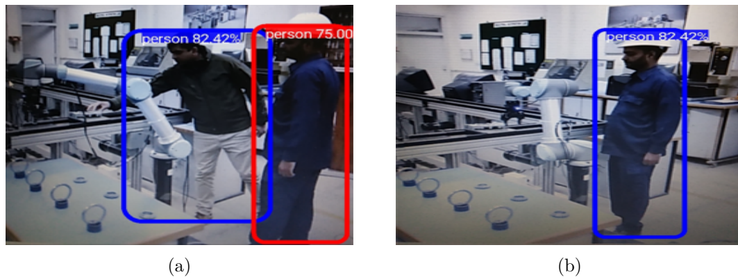
FIGURE 7.8: Detection and Action on Multiple Situations, (a) Detection of unidentified person and displaced case; (b) Picture showing the case being aligned by the cobot.
