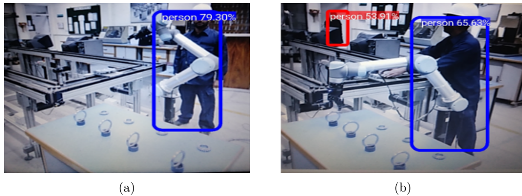
FIGURE 7.6: Recognition of Humans in Workspace, (a): Detection of Operator in Blue; (b): Detection of Unidentified Person in Red.
