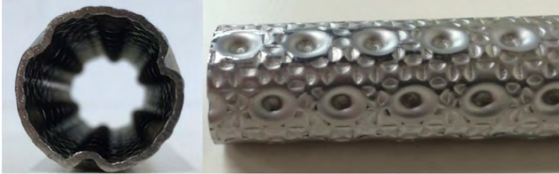
FIGURE 2.5: Dimple tube with rough surface [61]
