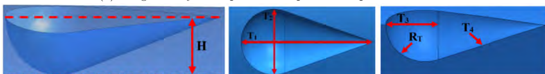
(b) 3D geometry of teardrop dimple with top and side views
